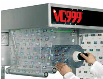
Top web infeed from above (integrated brake system)
