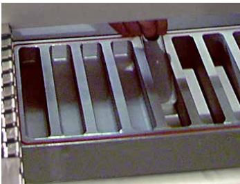
Forming station Rigid or flexible bottom web is heated and formed into pockets
