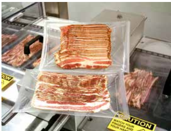
Sealing station Packages are evacuated, gas flushed (MAP) if required, and sealed
