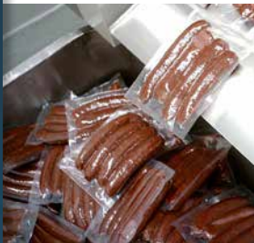
Cutting station Packages are separated Film trim is automatically removed
