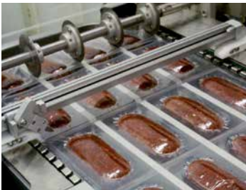
Cutting station Packages are separated Film trim is automatically removed
